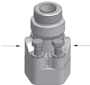
Push the flange clamps towards the flange head and screw fasteners into flange pad. Continue to screw the fasteners until their heads just meet the split flange surface.
