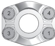
Torque the fasteners in diagonal sequence, in small increments, until final torque level is achieved. Torque values for flange connections listed above. Notice that the torque values vary according to size and fastener type.
